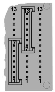
available for order. Thus any combination to connect an accupack can be realized. The third row of holes can be used to connect other plug systems by soldering the adapter cables to it. Although the UNI board can be used for different connecting systems, we recommend to use specifically configurated UNI boards for each application. Only this guarantees a maximum of safety.
