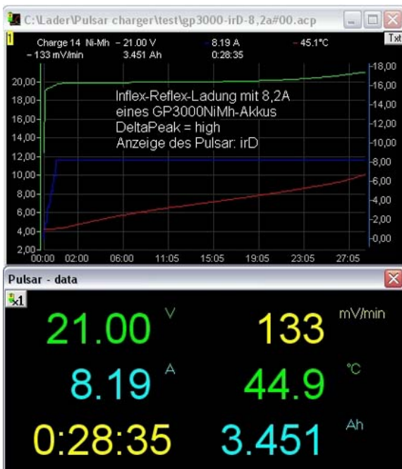
Charging of GP3000 pack in Inflex , Reflex with 8.2A
