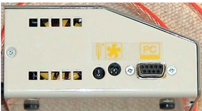
Left side: sockets for temperature sensor, external cooling fan and PC
