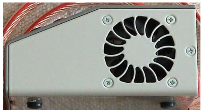
Right side: Laser cut intake for internal cooling fan
