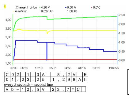
Charging ends when threshold voltage is detected and simultaneously charging current is decreased. When *Fast* mode is on charging current is controlled with pulses, which makes it possible to reduce charging time more than two times. Current limitation can occur when voltage overstep maximal value for given cell types. We recommend the *Pulsar EQUAL* Equalizer from ELPROG.
