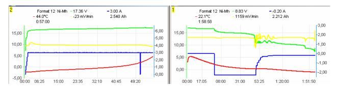
Formatting a battery means to perform demanded number (1 to 8) of discharging-charging cycles. Discharging is performed in *Auto* mode until threshold voltage is reached, which depends of cell type. Reconditioning a battery – special formatting mode which allows to repair the battery.
